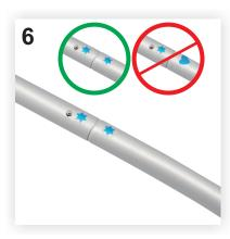
5-6. Applying the same method mentioned at pct. 1-2, add the corner items to the horizontal bars making sure to match the numbering / marking from the elements that merge, as in figures 5-6.
